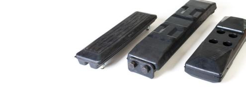
NTP rubber pads are available in three different versions; Chain-on which is replacing the steel shoe and bolted directly on the chain, Clip-on is attached with clips to the existing shoe, and Bolt-on which is bolted through pre-drilled holes
